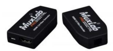
MuxLab 500464-V2 HDMI 2.0 Fiber Extender Kit enables the user to transmit 4K ( $4096 \times 2160$ ) video at 60Hz signal up to 1000m via OM4 multi-mode fiber, with any form of scaling or data compression being applied to the signal. This device supports a total data throughput of 18Gbps (6Gbps per lane). The unit supports HDR10+, Dolby Vision and HLG, as well as CEC, ARC, EDID and HDCP 1.4 & 2.2.
