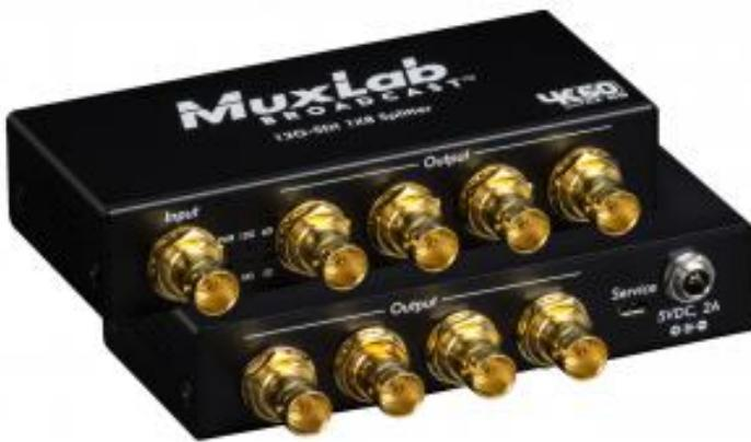
MuxLab 500728 12G-SDI 1x8 Splitter, 4K/60 allows one (1) 12G/6G/3G/HD/SD-SDI source to be distributed and amplified to up to eight (8) 12G/6G/3G/HD/SD-SDI displays. The splitter supports up to 4K (3840 X 2160) video and HD audio, including 480i (SD-SDI), 720p/1080i (HD-SDI), 1080p (3G-SDI), 4K/30 (6G-SDI) and 4K/60 (12G-SDI). The device automatically detects the 12G/6G/3G/HD/SD-SDI signal and re-clocks and regenerates the signal at the output for extending distances between source and displays.
