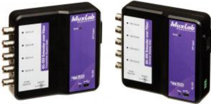
MuxLab 500732 6G-SDI Extender over Fiber Optic is a unique solution for extending SDI cameras or other SDI sources in up to 4K resolutions to a distance of up to 300m using OM3 fiber or up to 400m using OM4 fiber.
