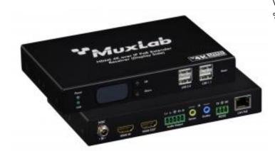
MuxLab 500850-RX KVM HDMI over IP PoE Receiver allows HDMI & USB equipment to be connected up to 100m over an Ethernet LAN, supports HDMI up to 4K @ 30Hz (4:4:4) and 4K @ 60Hz (4:2:0) via Cat5e/6 cable in multiple point-to-point and point-to-multipoint configurations. The Transmitter (500850-TX) and Receiver (500850-RX) support PoE (PD) if used with a PoE (PSE) Ethernet Switch.
