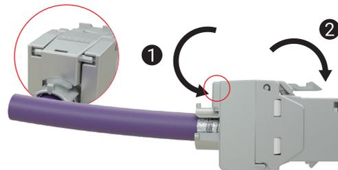
9. Close latch in two steps. Lugs must be in notches as shown above.
