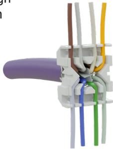
6. Cut off excess wires, taking care to cut flush to the wire manager.
