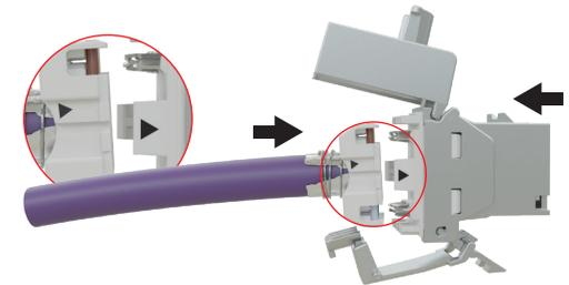
7. Insert wire manager into keystone body, ensuring that the arrow on both are aligned on the same side.
